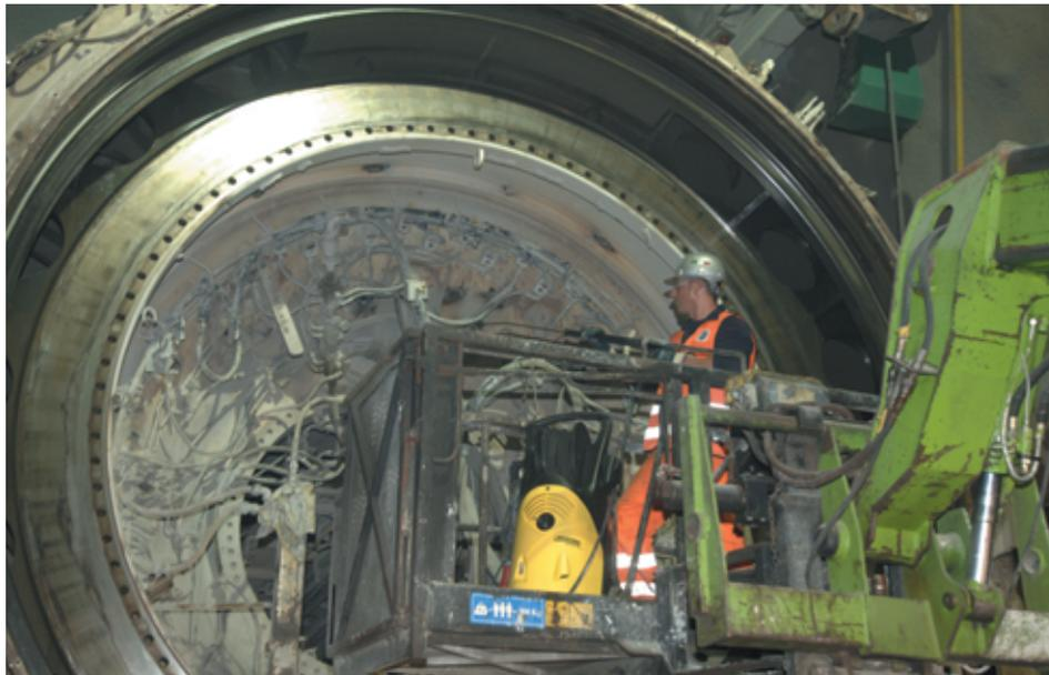
dozens of pressure washers in the tunnels and at each portal. Bright yellow Kärcher washers make a striking contrast in the grey and tawny world deep inside the Alps. Everything has to be washed – all external surfaces of the TBMs including the cutting discs as well as conveyors and concrete pumps, along with all manner of mobile equipment outside the tunnels where temperatures vary seasonably from hot to bone-chilling cold.
