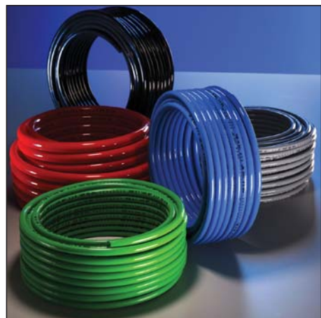
Polyurethane hoses from LEONI EPS are constructed of a fibre braid reinforcement sealed between two extruded PUR layers.
