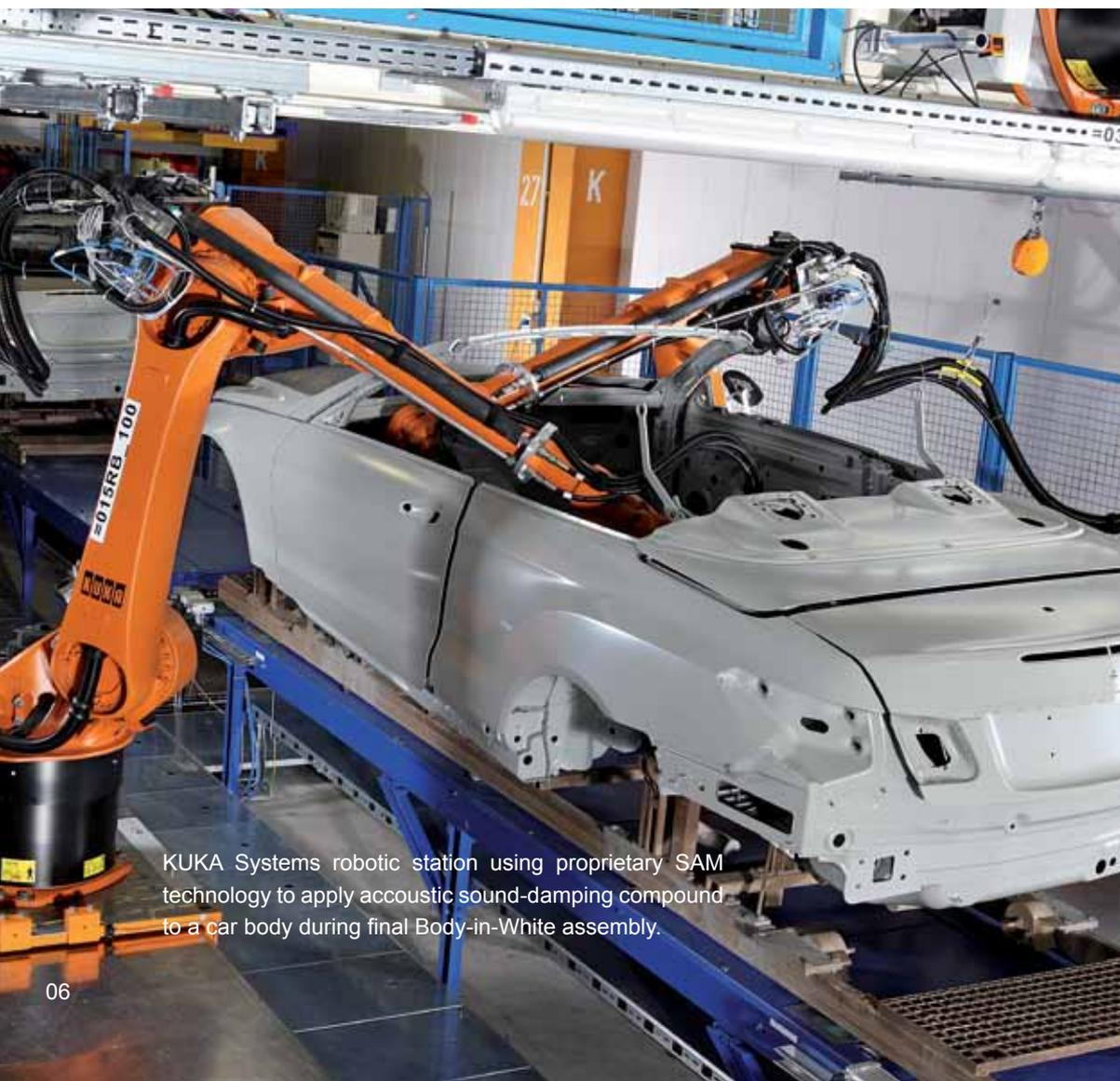
KUKA Systems robotic station using proprietary SAM technology to apply acoustic sound-damping compound to a car body during final Body-in-White assembly.
