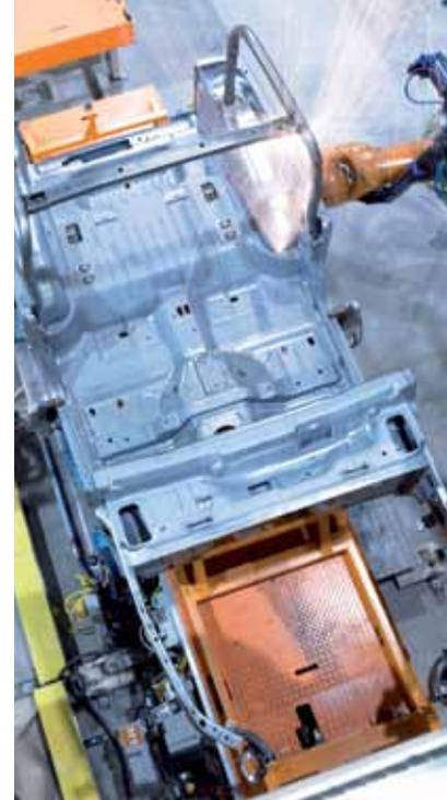
KTPO has a worker/robot ratio of 1:1. Of its 245 robots, 68 perform materials handling, 166 welding tasks and 11 roller hemming.
