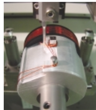
Figure 2: Core winding facility at TransERA-plant in Waterloo.
